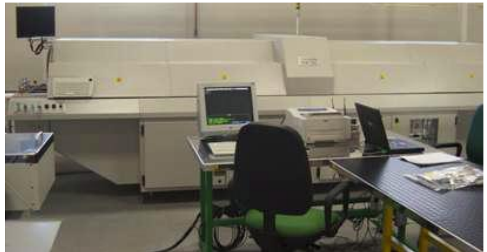
Oven for Soldering Reflow – 14 zones
